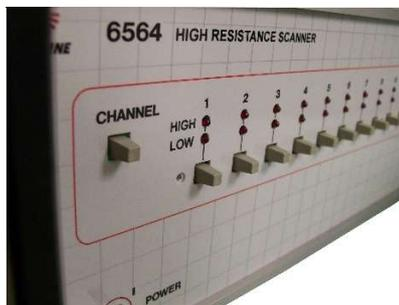
never previously been commercially available, and will greatly improve the measurement and calibration throughput of high and ultra-high ohm resistors now that standard laboratories can easily and quickly **automate single and multiple** high to ultra-high resistance measurements. The 6564 Series Scanners provides **>10<sup>17</sup> isolation**, measurements to 10 P $\Omega$ , and with voltages up to 1000 V with no guarding required!
