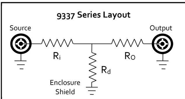
$R_i$  and  $R_o$ ) to give the desired nominal value. This design provides for a **very high quality and stable** standard and is **not as reactive to environmental** parasites as typically found in other high value resistance standards. This configuration (shown left) is also sometimes referred to as a delta-wye configuration.
