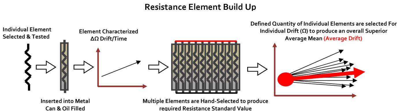
The multiple elements are sealed in epoxy for protection against humidity, are bonded to a thermal block, and are placed into the provided EMI shielded outer case with high quality gold plated terminals attached.
