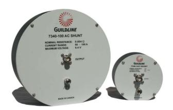
Current Shunts can be used for a variety of AC/DC current measurement applications and have a nominal impedance range of 100  $\Omega$  to 0.004  $\Omega$ . The frequency bandwidth of this series is 100 kHz for all current outputs. For low currents a buffer amplifier is available.
