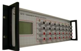
**New Thermometry Adapter**: The new Guildline 3210 Thermometry Adaptor, and optionally a Low Thermal Matrix Scanner, is included with the System. Every one of the eight channels on the model 3210 Thermometry Adaptor has its own pre-warm capability and automation support. The channels in pre-warm are identified with a yellow LED indicator while the selected channel being measured has an active Green LED indication.
