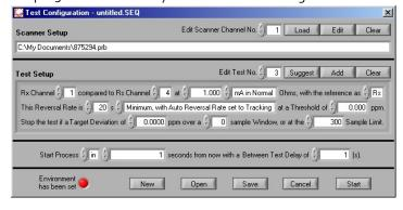
**BridgeWorks** software offers many routine **thermometry functions such as SPRT calibrations** to ITS-90 scale. It also provides comprehensive graphic display, math functions and trend analysis. Data can be **easily exported** to MS-Excel®, Crystal Reports®
