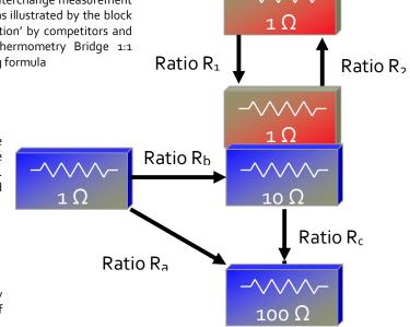
This **Multi-Ratio** capability allows users to extend the calibration interval of the Thermometry Bridge while still maintaining a high level of confidence, thus saving thousands of dollars each year in support of the instrument. With an annual verification, a Guildline 6622T Thermometry Bridge typically can go five years between calibrations.
