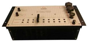
terminal shunt. The design optimizes a number of important factors such as the effects of self-heating, temperature coefficient, size, weight, ease of operation and total measuring range. They provide wide range precise current measuring capability when used with a potentiometer or digital voltmeter as a readout.
